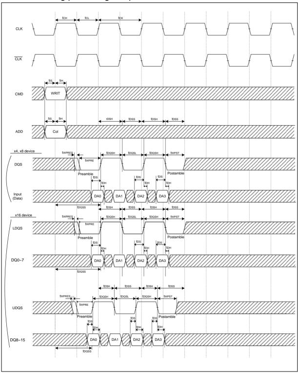
Note: x16 has two DQSs (UDQS for upper byte and LDQS for lower byte). Even if one of the 2 bytes is not used, both UDQS and LDQS must be toggled.
