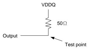
Figure 2: Pulldown slew rate test load
