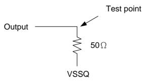
Figure 1: Pullup slew rate test load
