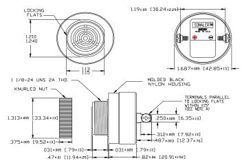
NOTE A: TERMINALS-032 BRASS TIN PLATED, TAPPED FOR #6-32 SCREW. TWU #6-32 NICKEL PLATED BRASS SCREWS INCLUDED, WILL ACCEPT 1/4\* QUICK CONNECT. NOTE B: MOUNTING- REMOVE BLACK PLASTIC NUT AND INSERT THREADED FRONT THROUGH 1.25' HOLE PUNCHED IN PANEL, IF DRIENTATION IS NEEDED, NOTE LOCKING FLATS ON DRAVING. SCREW NUT BACK ON. DO NOT OVERTIGHTEN.
