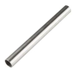
**Description:** These 10" long stainless steel tubes have an outer diameter of 1", an inner diameter of 0.88", and a wall thickness of 0.06". When used with the mating tube clamps, these can be used for versatile structural support. Additionally, wires and cables can easily be run through the center.
