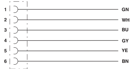
Contact assignment of 7/8" socket
