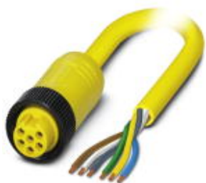
Power cable, 6-position, PVC, yellow, free cable end, on Socket straight 7/8"-16UNF, cable length: 10 m
