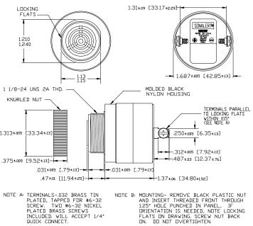
NOTE B: MOUNTING- REMOVE BLACK PLASTIC NUT AND INSERT THREADED FRINT THROUGH 1.25' HOLE PUNCHED IN PANEL, IF DRIENTATION IS NEEDED, NOTE LOCKING FLATS ON DRAWING. SCREW NUT BACK ON. DO NOT DVERTIGHTEN.
