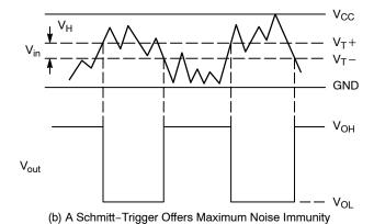
Figure 6. Typical Schmitt-Trigger Applications
