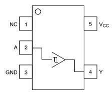
Figure 1. Pinout (Top View)
