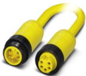
Power cable, 5-position, PVC, yellow, Plug straight 7/8"-16UNF, on Socket straight 7/8"-16UNF, cable length: 2 m
