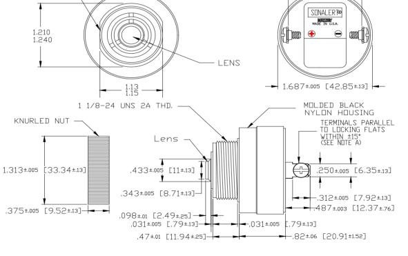
NOTE A: TERMINALS-.032 BRASS TIN PLATED, TAPPED FOR #6-32 SCREW. TWO #6-32 NICKEL PLATED BRASS SCREWS INCLUDED. WILL ACCEPT 1/4" QUICK CONNECT. NOTE B: MOUNTING- REMOVE BLACK PLASTIC NUT AND INSERT THREADED FRONT THROUGH 1.25" HOLE PUNCHED IN PANEL, IF ORIENTATION IS NEEDD, NOTE LOCKING FLATS ON DRAWING. SCREW NUT BACK ON. DO NOT OVERTIGHTEN.
